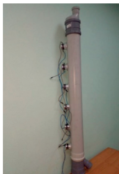
Figure 2 Experimental stand of the ultrasonic muffler of a Diesel engine
