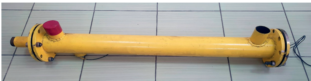
Figure 2 Full-size ultrasonic vehicle muffler bench
