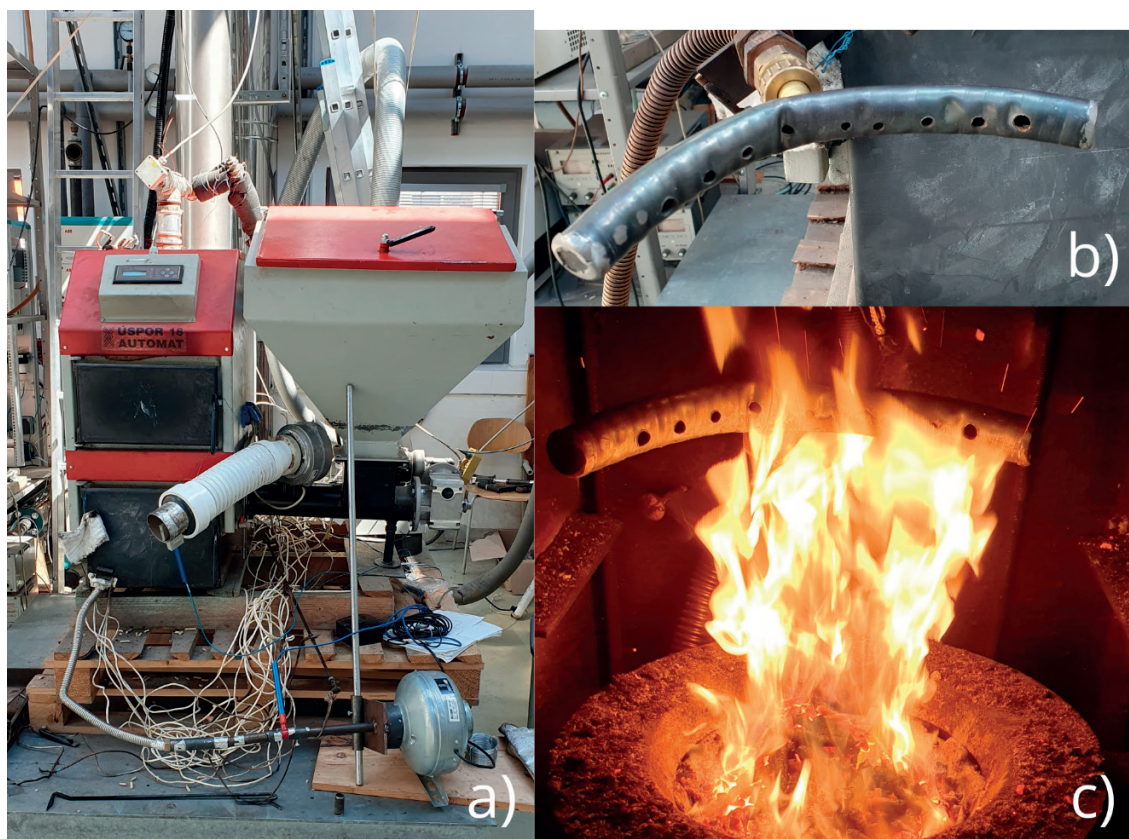
Figure 3 Real experimental setup for the tertiary air supply: a) overall system, b) air duct detail, and c) combustion chamber view
