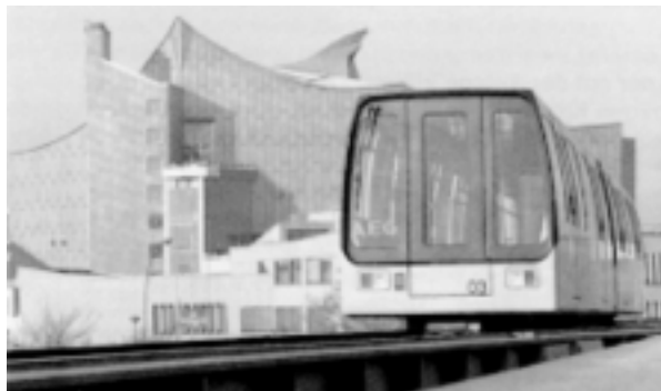
Fig. 1. Maglev-vehicle MAGNETBAHN Berlin [1]
