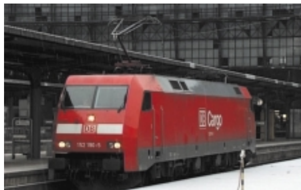
Fig. 8. Class 152 heavy duty locomotive (86 t, 140 km/h, 6.4 MW), which could be equipped with boosters
