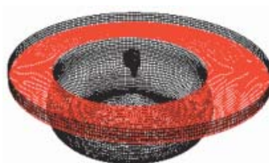
Fig. 4 Surface grid of combustion chamber without the engine head grid
