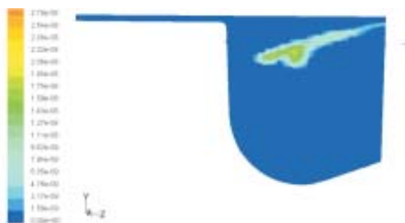
Fig. 29 Droplets of ethanol (kg/s) -10 °CA before TDC, kinetic model
