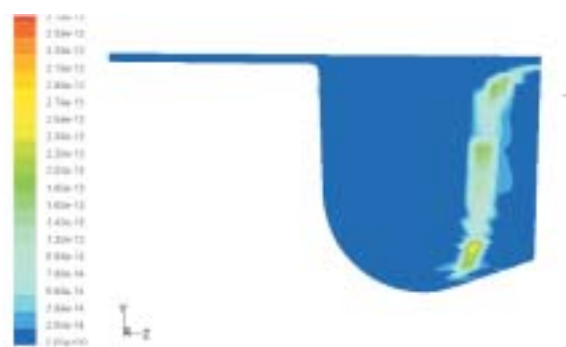
Fig. 32 Droplets of ethanol 5 °CA after TDC, kinetic model
