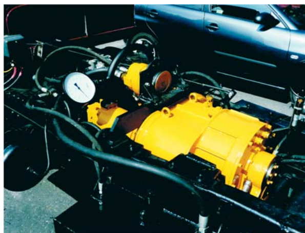
Fig. 4. The IVT 150 installed to the truck frame
