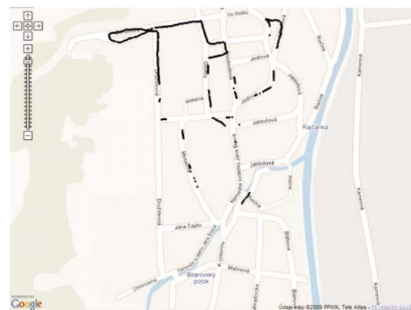
Fig. 4 Radio map database filtered for BS with CID=4F81, BSIC=29 and BCCH=15
