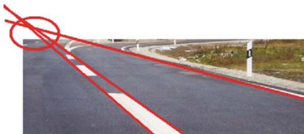
Fig. 3 Position Estimation: Determining the vanishing point and using landmarks
