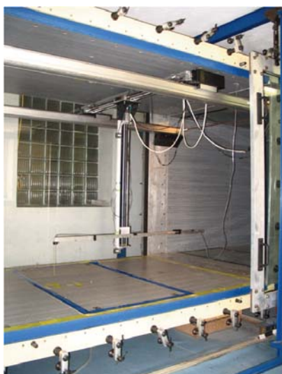
Fig. 1 Gauge section of the aerodynamic tunnel
