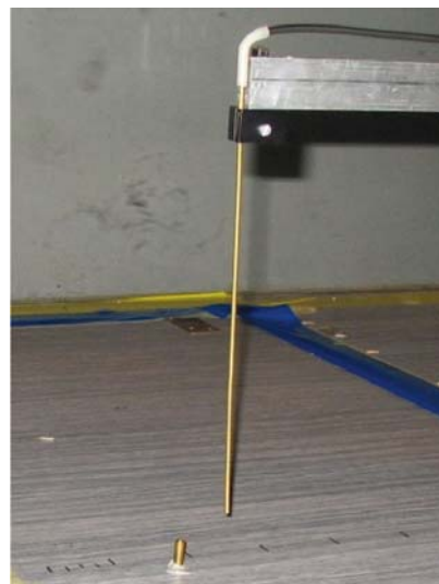
Fig. 3 Pollutant source on the floor and measuring probe
