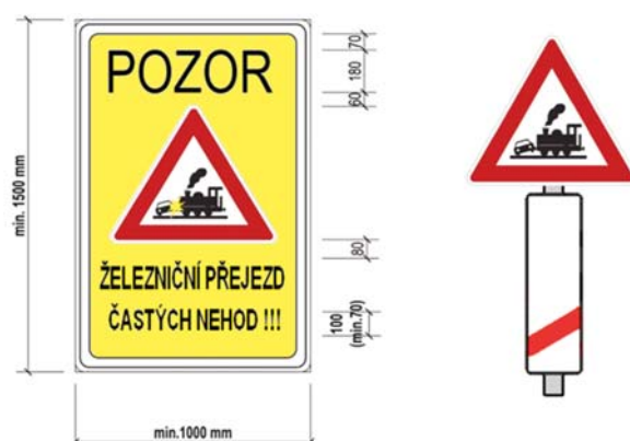
Fig. 2 Design of traffic sign “Caution, frequent accident level crossing”
