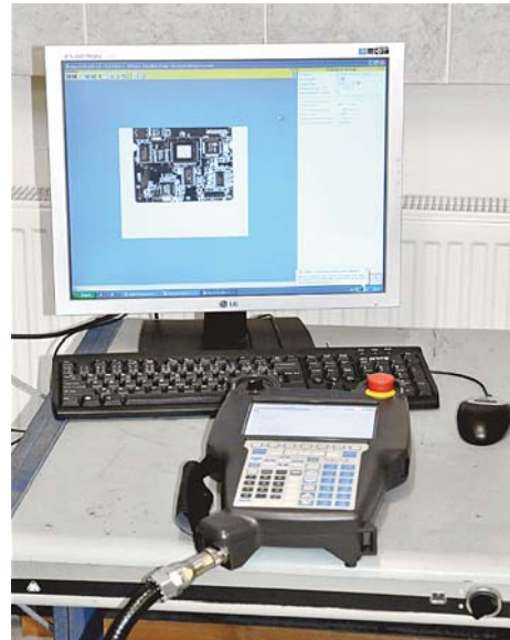
b) Control system include the Vision Tool and so-called teach-pendant
