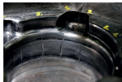
Fig. 5 Fatigue cracks on the functional surface of die forging
