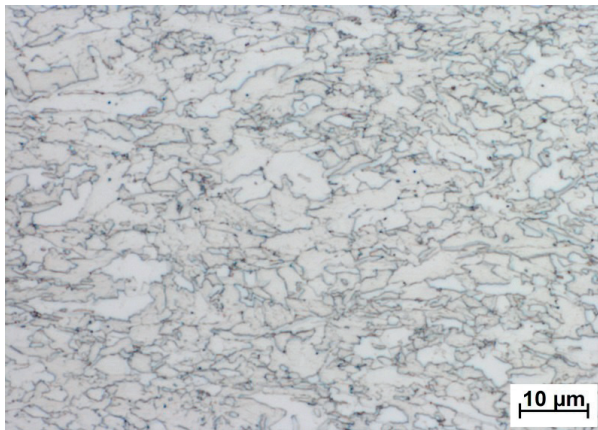
Fig. 1 Microstructure of tested steel STRENX 700MC
