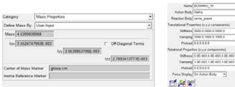
Figure 6 Mass settings and stiffness of elements in ADAMS
