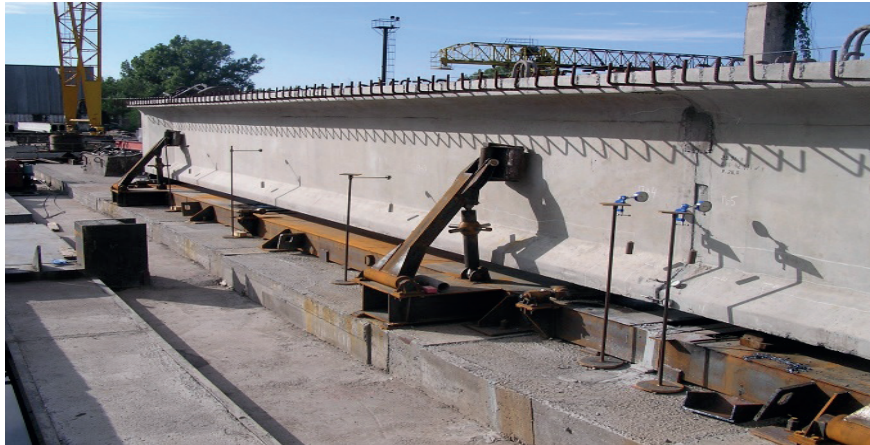
Figure 14 Fragment of a 42.0 m long composite beam with mounted deflectometers and clock type indicators
