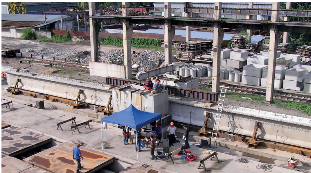
Figure 14 Fragment of a 42.0 m long composite beam with mounted deflectometers and clock type indicators
