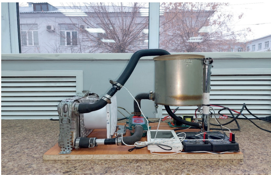
Figure 5 experimental bench for ultrasound cleaning the car radiator
