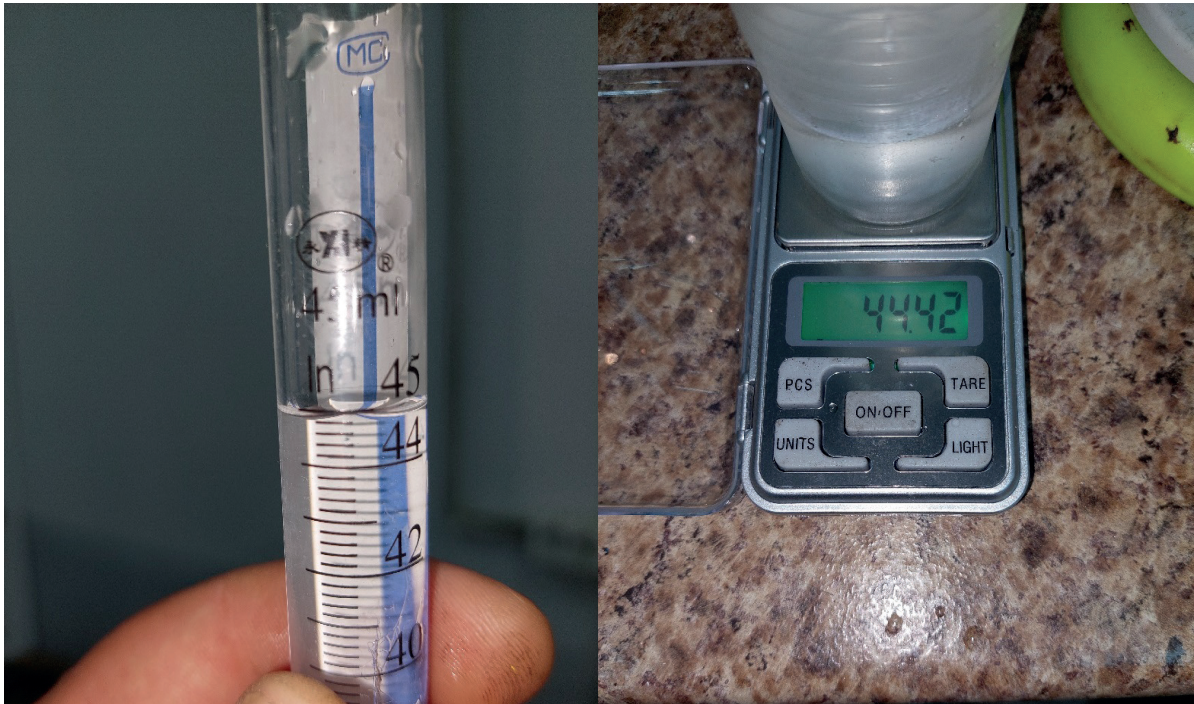
Figure 8 Determining the liquid volume using a volumetric flask and the mass of liquid on the balance
