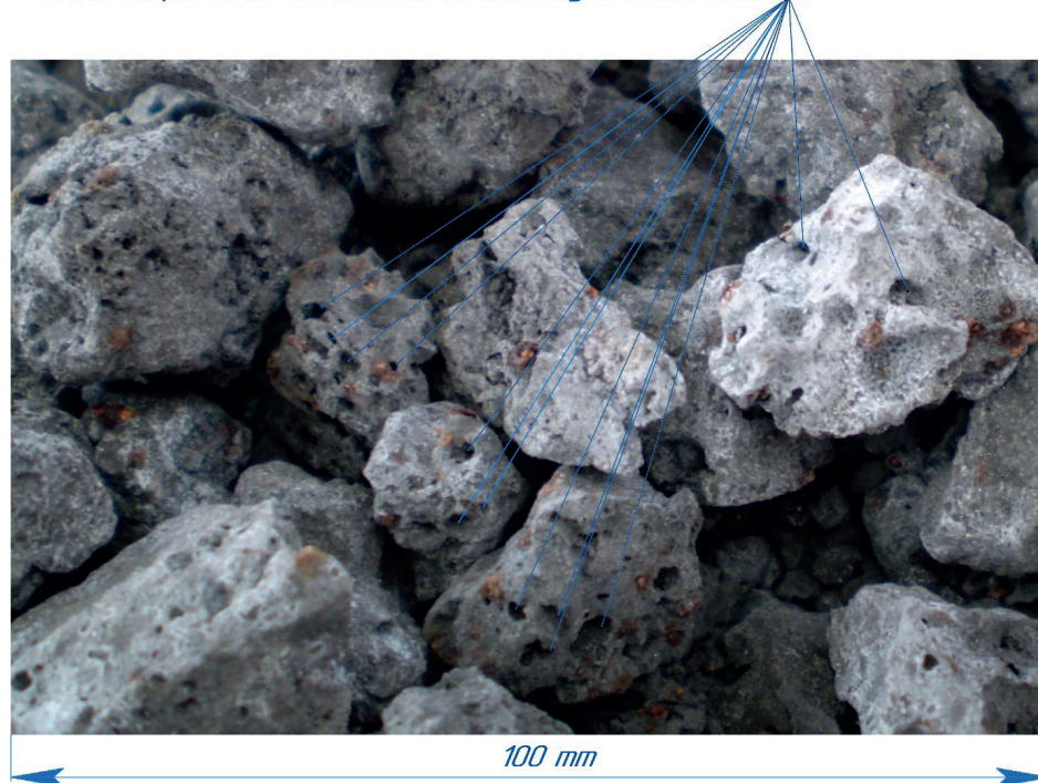
Figure 2 External pores on the surfaces of slag crushed stone grains
