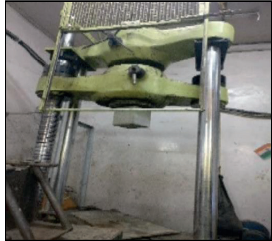
Figure 4 Pull-out test (a) Specimen details (b) setup
