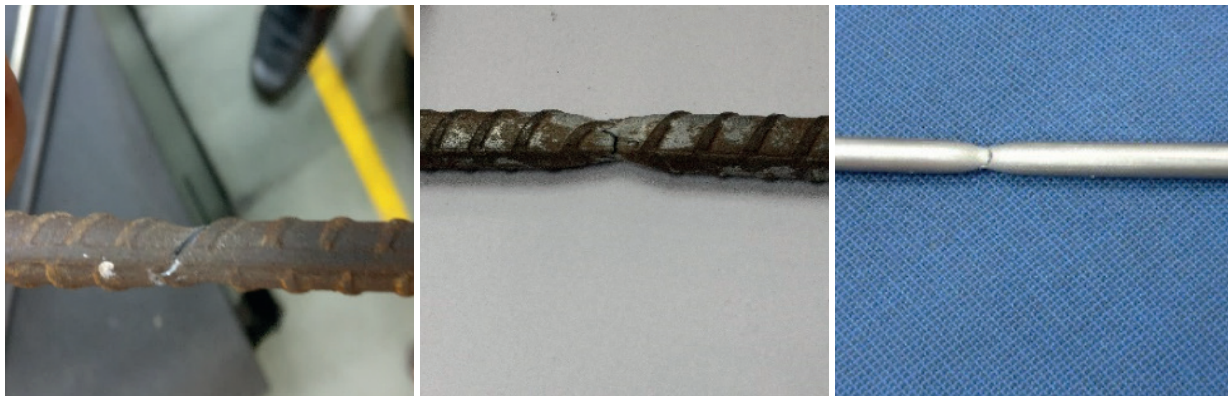
Figure 8 Specimen after the tensile test (a)mild steel (b) TOR steel (b) Fe-SMA
