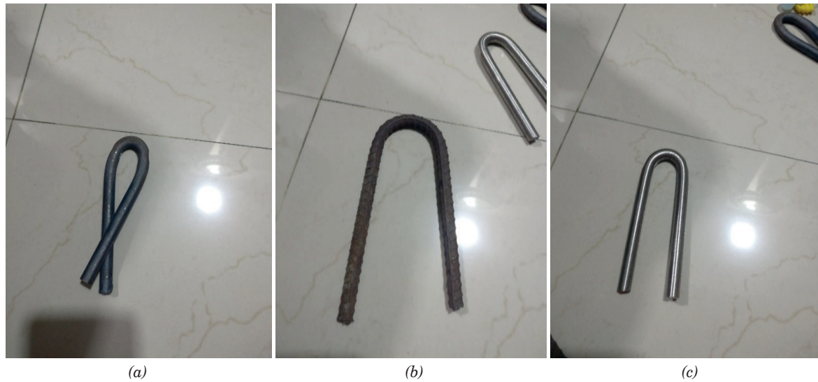
Figure 9 Specimens after bend test (a) mild steel (b) TOR steel (c) Fe-SMA
