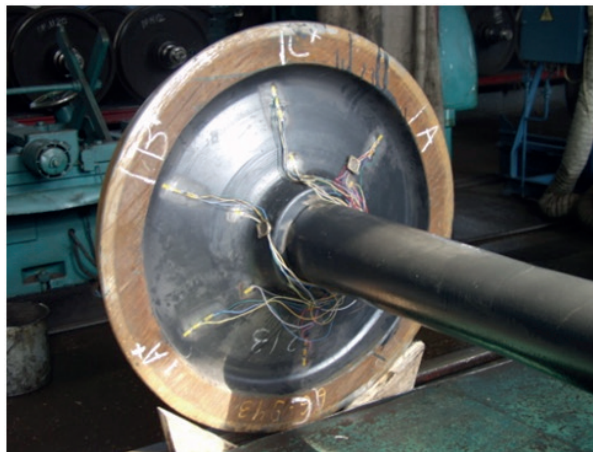
Figure 8 Measuring scheme on the experimental wheel pair
