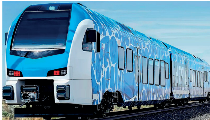
Figure 3 An illustration of the multiple unit by Stadler known as Flirt H2 [41]
