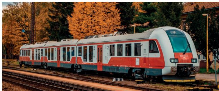
Figure 4 The multiple unit 861 class produced by the ZOS company originally powered by diesel powertrain [42]
