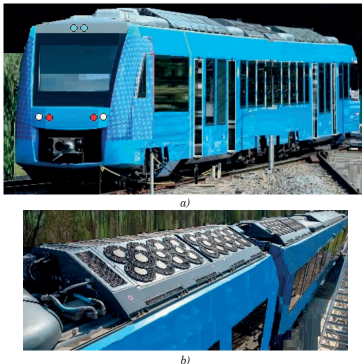
Figure 1 a) A multiple unit by Alstom equipped by hydrogen fuel powertrain known as Coradia iLint, b) an illustration of a layout of the components of the hydrogen powertrain on a vehicle roof [39]
