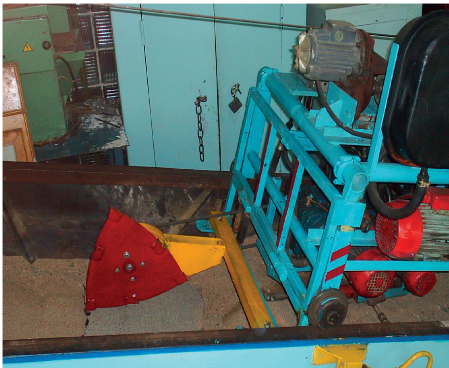
Figure 3 Experimental setup with cycloidal motion of the working body
