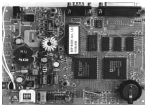
Fig. 1. IGC unit - view from component side
