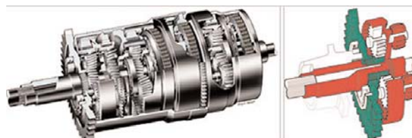
Fig. 1: Agrottron TTV gearbox cross section and detail of the power split point
