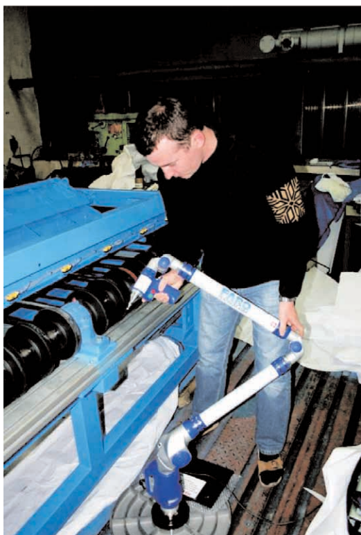
Fig. 8 Measuring of the object with FARO
