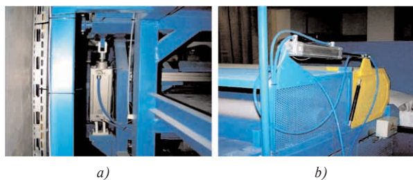
Fig. 13 a) pneumatic cylinder – loader b) pneumatic cylinder – cover
