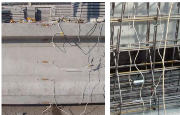
Fig. 4b) Strain gauges and elastomagnetic sensors
