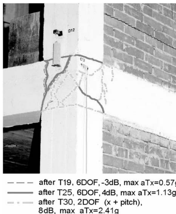
Fig. 10 Cracks in critical sections of R/C frame at the end of test - frame joint at the first floor
