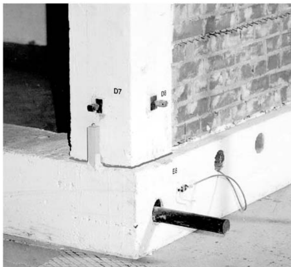
Fig. 11 Cracks in critical sections of R/C frame at the end of test - frame joint at the base
