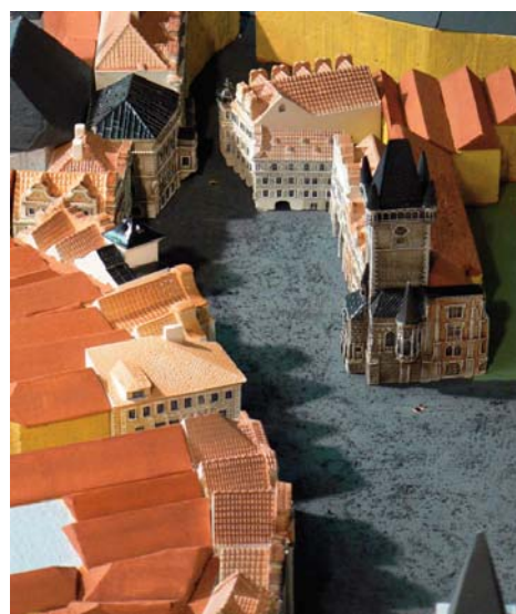
Fig. 1: Model of the Old Town Square in the aerodynamic tunnel [Source: own]
