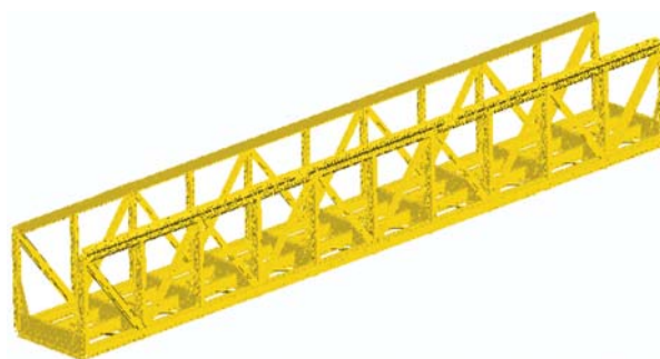
Fig. 4 Cross-section of the observed railway truss bridge and its computational model
