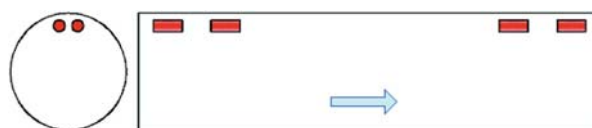
Fig. 6 Combined connection of 4 \times 2 parallel fans, variant c
