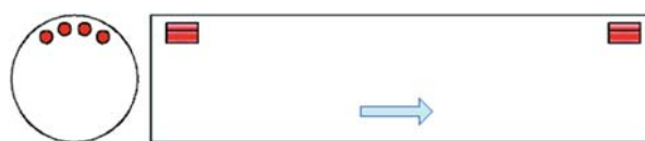
Fig. 5 Combined connection of 2 \times 4 parallel fans, variant b
