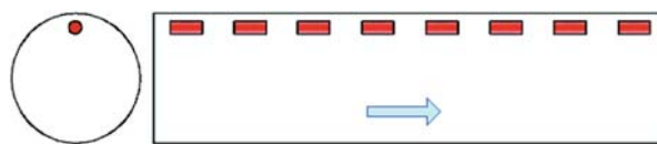
Fig. 7 Serial connection of 8 fans, variant d
