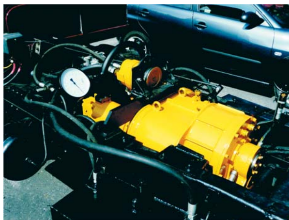
Fig. 4. The IVT 150 installed to the truck frame
