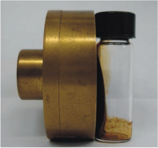
Fig. 2 Encapsulated taxol and MF-PEG in PLGA attached to a magnet
