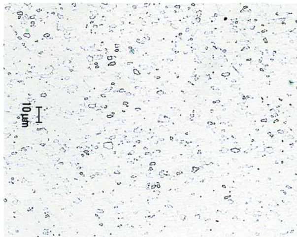
Fig. 1 Microstructure of steel sheet H220YD
