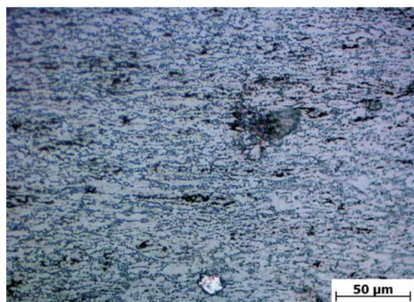
Fig. 1 Microstructure of Ti6Al4V alloy, etched 2 mL HF+8 mL HNO 3 + 90 mL H 2 O [9]
