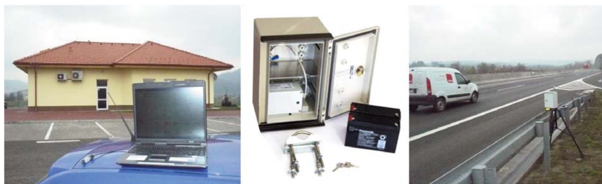
Fig. 1 Automatic system for traffic intensiveness monitoring (SIERZEGA SR4)
