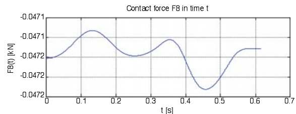
Fig. 6 Time course of the contact force F8 under rear wheel of the rear axle
