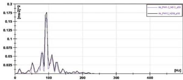
b) LABVIEW Analysis: The PWS of the ballast bed acceleration w''_B(t) /the accelerometer A_B , the passage of coach bogies No.1-2, t = 3.01 - 3.8 = 0.79 s.
