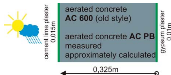
Fig. 3 Scheme of the analyzed building's envelope
