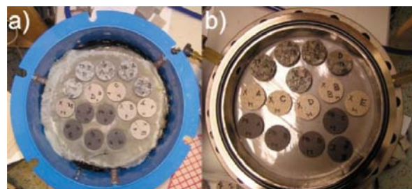
Fig. 6 a) pressure plate extractor PPE, b) pressure membrane extractor PME before setting pressure level
