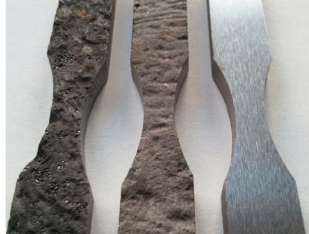
Fig. 2 Surface condition of specimens (from left as-cast, sand blasted, fine ground)
