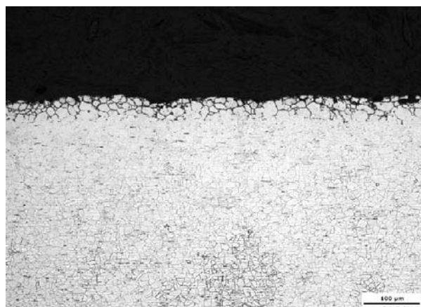
Fig. 6 Damage of the AISI 316Ti after 1 year exposition in the duct system outlet (a), mag. 400, and after 30 days in the duct system inlet (b), mag. 200, etch. Rollings
