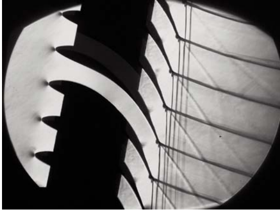
Fig. 4 The schlieren picture of the flow field in a profile cascade, \alpha = 0^\circ , M_{2is} = 1.828 . No additional shock waves visible, perfect flow field periodicity in exit part of interblade channels
