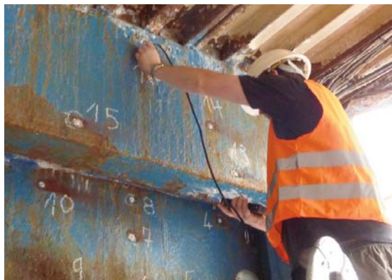
Fig. 2 Experimental measurements of the section thickness of Beam 6 in the most exposed locations
