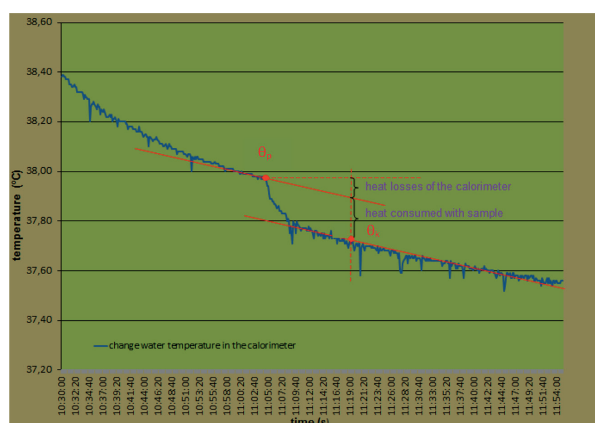
Fig. 3 Graphic record of the calorimetric test of the sandy gravel layer and the method of its evaluation
