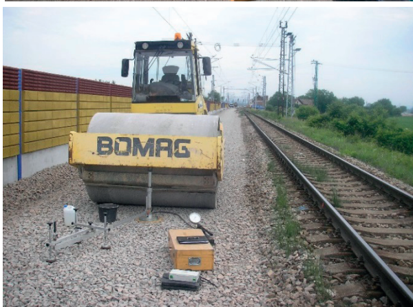
Fig. 9 Implementation of the static loading test in the northern portal (left on the surface of frost-resistant protective layer in the area of slab track, right on the surface of the railway ballast in the area with standard structure of railway superstructure)
