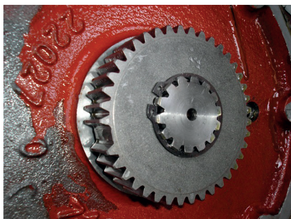
Fig. 6 Sun gear with one missing tooth
