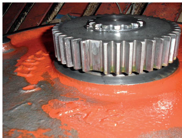
Fig. 6 Sun gear with one missing tooth
