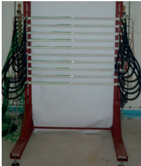
Fig. 4 Arrangement of pipes in a thermostatic chamber at axial distance of pipes 5D [6]
