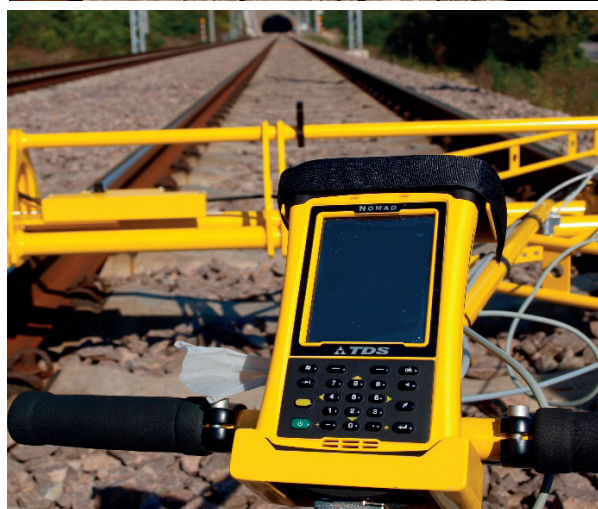
Fig. 2 Continuously measuring trolley KRAB TM -Light (on the up) and computer Nomad (on the down)
