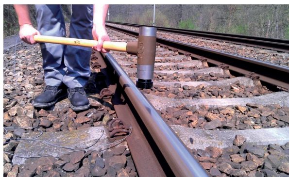
Fig. 2 The test in-situ, impact excitation
