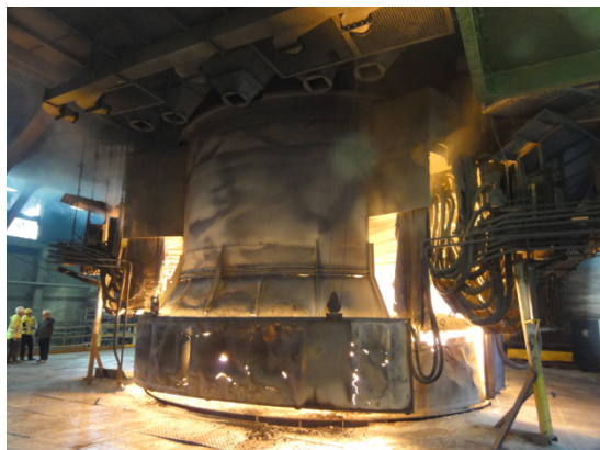
Fig. 2 ARC furnace used for ferroalloy production in OFZ, a.s. Istebne, plant Siroka
