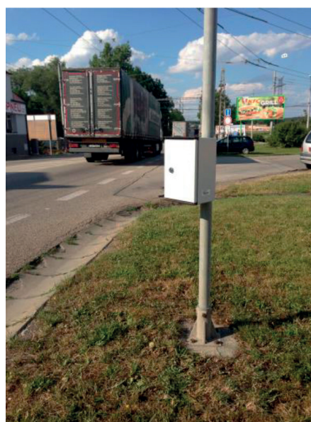
Fig. 1 Sierzega SR4 device mounted on the post of road sign - suitable for long-term measurements (source: Authors)
