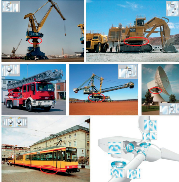
Figure 1 Examples of the slewing bearings applications
