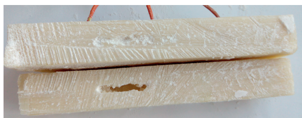
Fig. 9 Shrinkages and cavities in the samples
