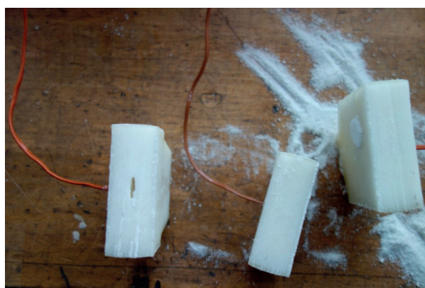
Fig. 8 Sample after removal from the ingot mould and slicing
