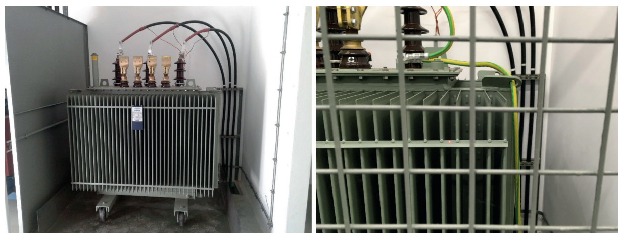
Figure 4 Tested HV transformer; without the safety barrier (left), measuring points programming (right)
