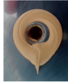
Figure 9 Result of paste application along the circular path.
