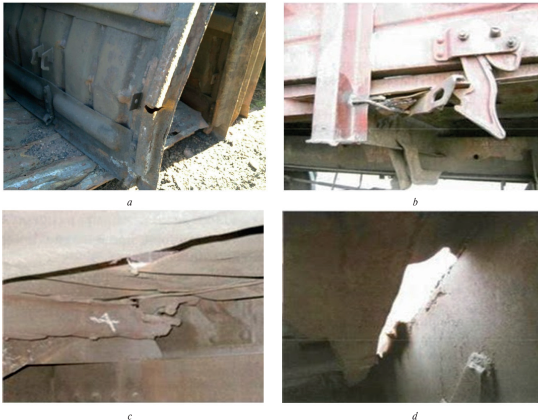
Figure 1 The basic damages in the hatch covers of open wagons in operation: a - break in the framing, b - tear of the locking support, c - damages in the framing, d - tear of the sheet
