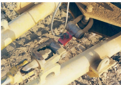
Figure 3 Tractive power registration
